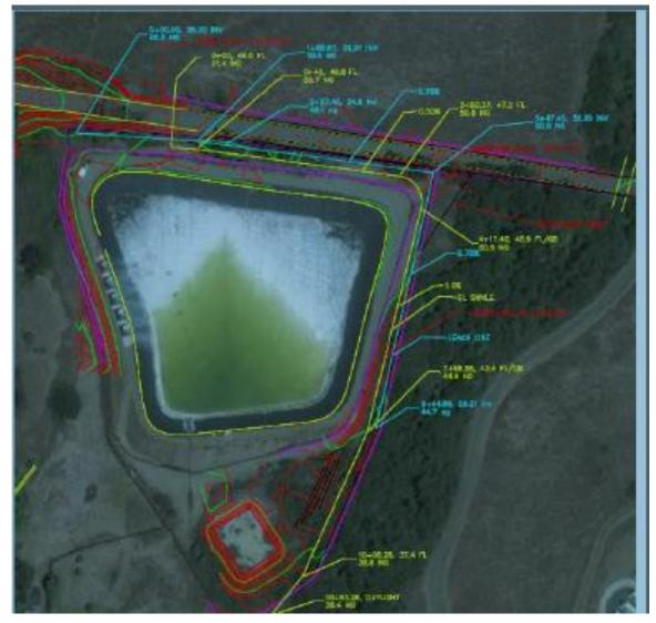
Yellow line work depicts swale alignment and grade. Blue line work is not in the contract. Swale to have 8 foot wide bottom with 2:1 sloped sides or flatter. Swale shall be lined with North American Green BioNet SC150BN.
